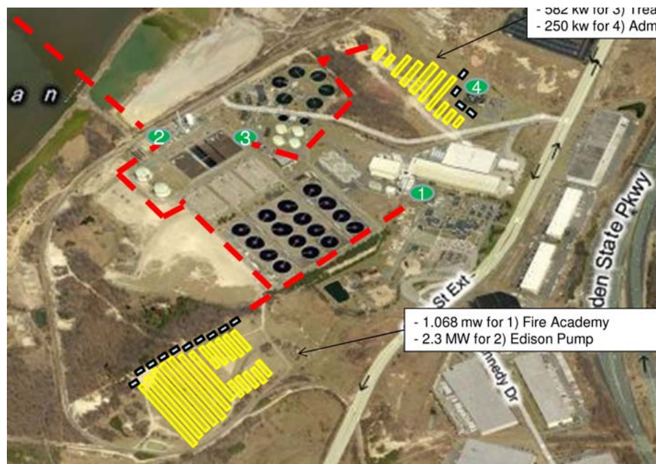
Proposed solar panel areas at the MCUA; actual locations may differ slightly.
